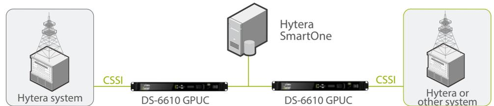
**Typical case:** The Urban area adopts a DMR Trunking system, while the suburbs adopt DMR Tier 2. Via Hytera SmartOne, the two systems can be connected seamlessly; terminals can roam between these two systems and be contacted via a common dispatcher.
